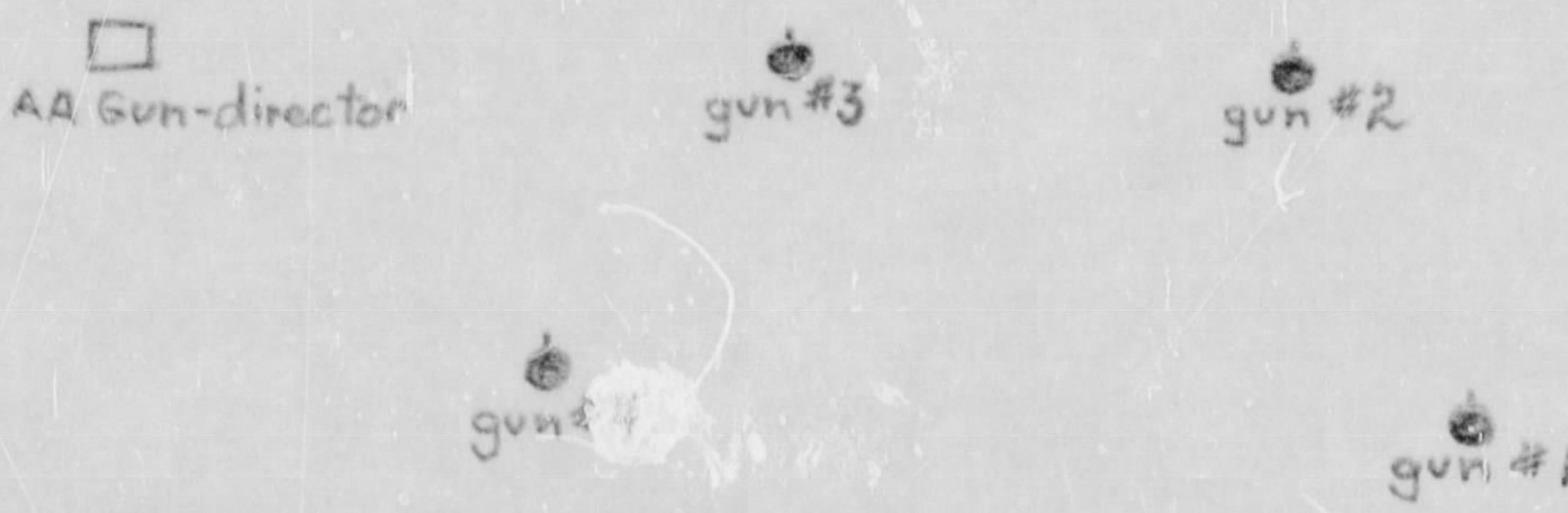
that in delivering fire on ground targets, there will be a minimum of interference between guns. The gun-director should be located forward and somewhat to the side.
